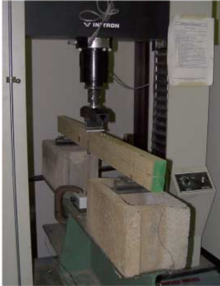
Figure 4.1 3-Point Flexure Test Setup with String Gage.
