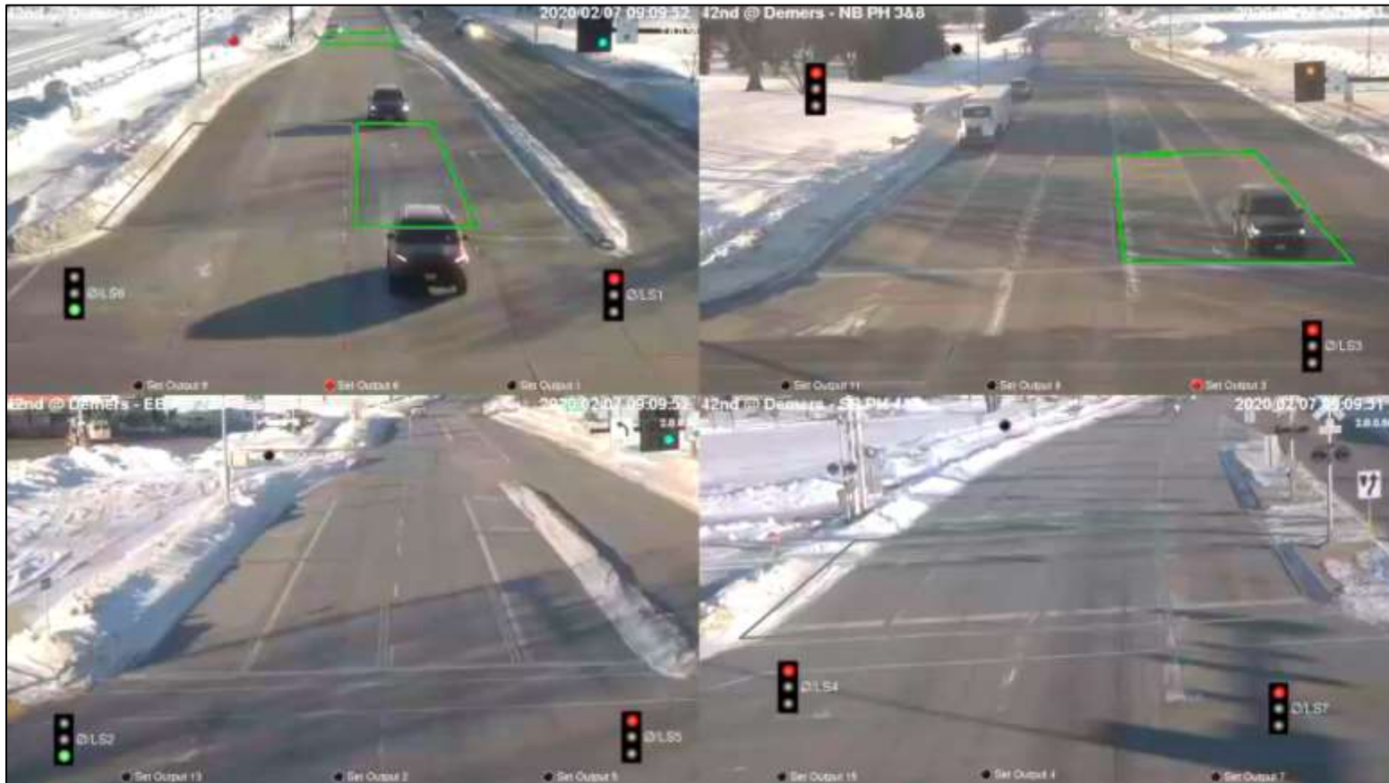
Figure 7. S 42nd St. at Demers Ave. EB camera in-and-out of low detail mode
