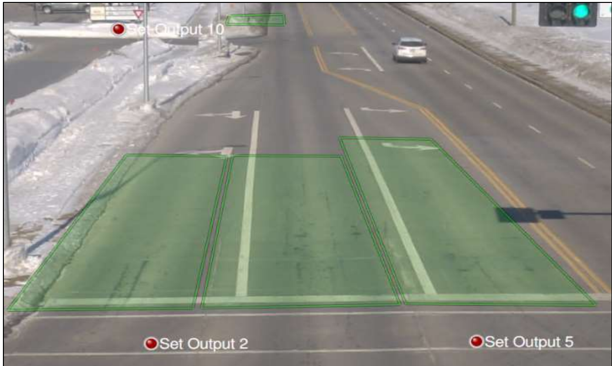
Figure 3. Existing zone setup for N 42nd St. at University Ave. southbound
