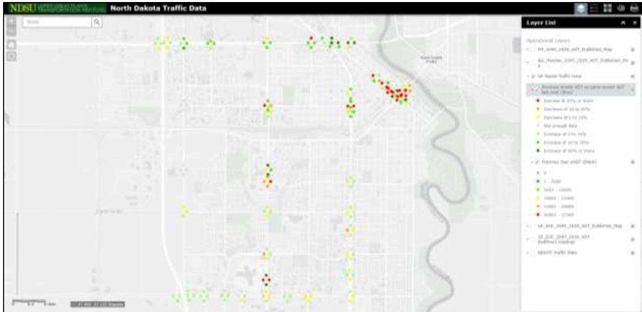
Figure 11. Sample of color-coded traffic changes at Grand Forks intersections on ND Traffic Data Portal
