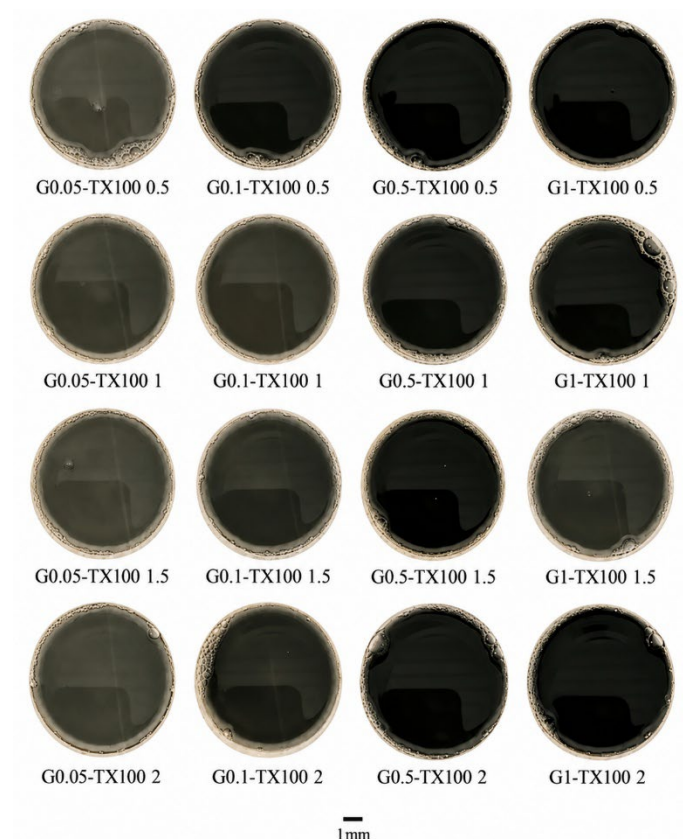
Figure 11. Images of GNP dispersions prepared with TX-100 at different TX-100-to-GNP ratios and GNP concentrations. Rows correspond to TX-100-to-GNP ratios of 0.5, 1.0, 1.5, and 2.0, respectively. Columns correspond to GNP concentrations of 0.05%, 0.1%, 0.5%, and 1.0%, respectively.
