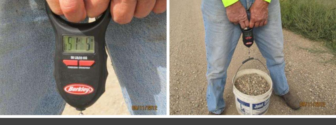
Simply remove loose aggregate from a 10 inch cross section, weigh it and convert that to a one-mile section
