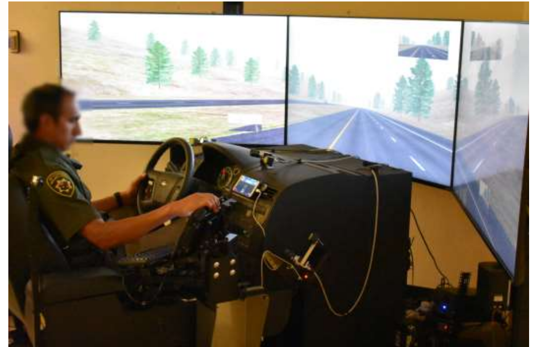
High Fidelity Car Simulator – WYOSAFESIM University of Wyoming
