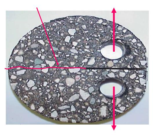
Motivation – measure fracture energy, use cylindrical specimens, maximize repeatability, use true fracture test
