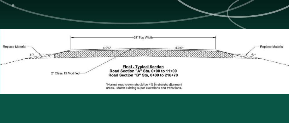
302-P01 AGGREGATE SURFACE COURSE CL13: Aggregate Surface Course CL 13 shall be placed after full depth reclamation and surface is shaped to 4% normal crown. Aggregate quantity is estimated at 37.4 Tons per Station. An additional 704 Tons is included for approaches.
