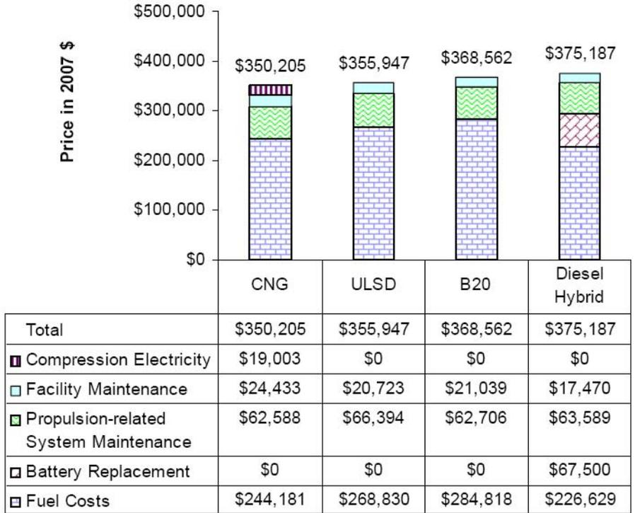
**Figure 8.4** Average Operating Cost per 40-foot Bus in a 100 Vehicle Fleet
