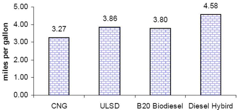
**Figure 8.5** Average Fuel Efficiency in Standard 40-foot Bus
