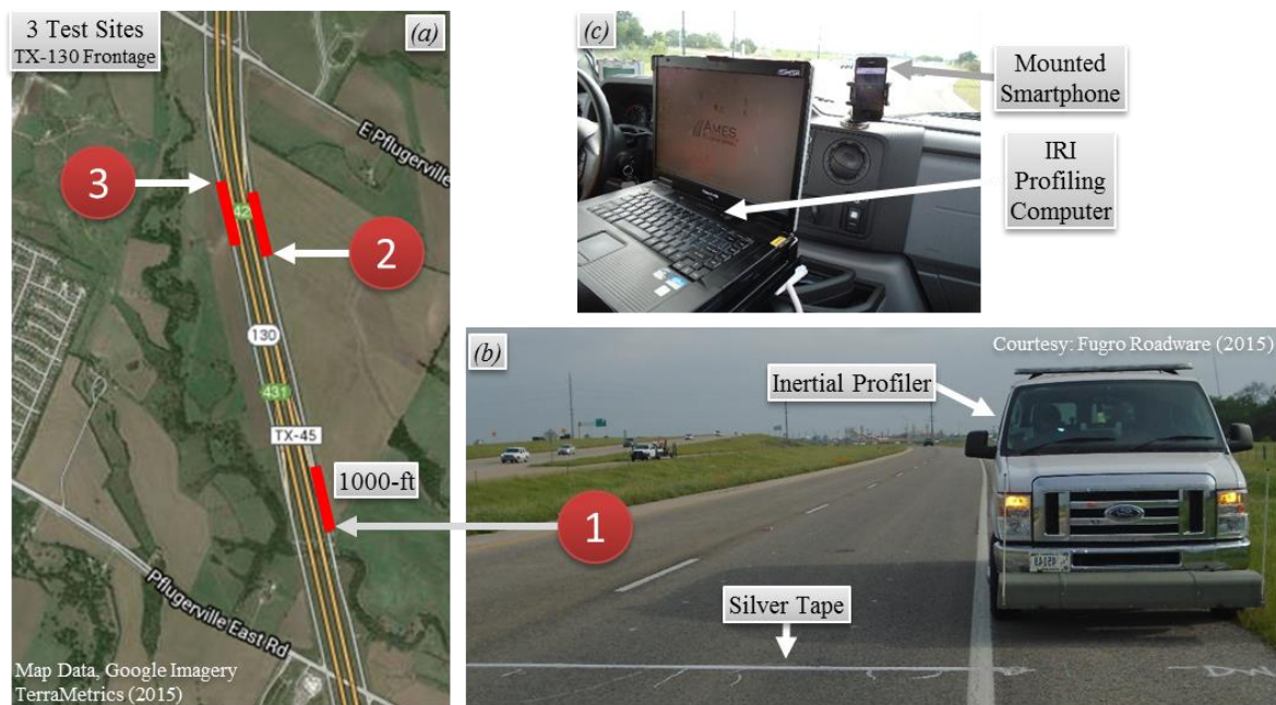
FIGURE 2 The roadway sections analyzed.
