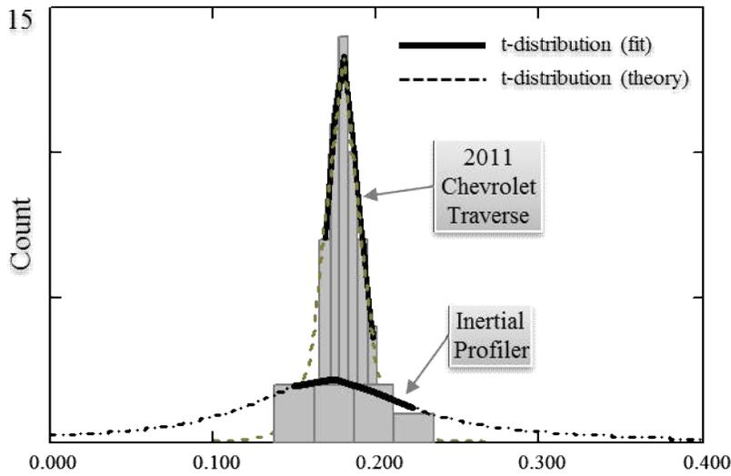
Figure 2. Distribution of RIF-indices from each vehicle for the 70-meter segment.
