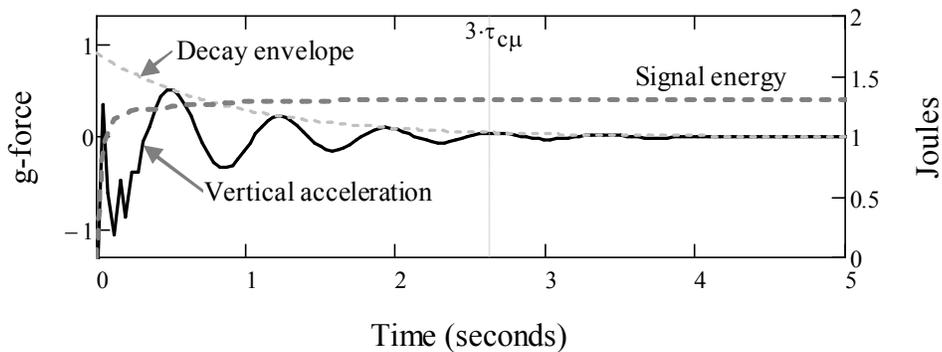
Figure 2. Simulated vertical acceleration of the suspension impulse response and signal energy
