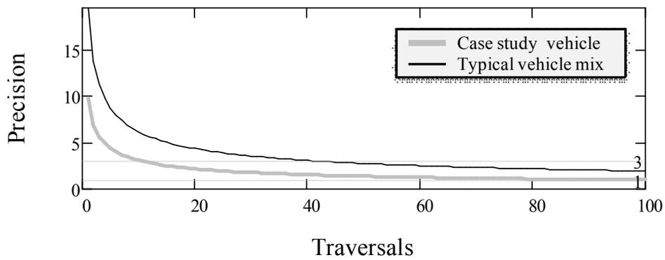
Figure 8. Precision bounds for the speed bump case study vehicle and an expected vehicle mix
