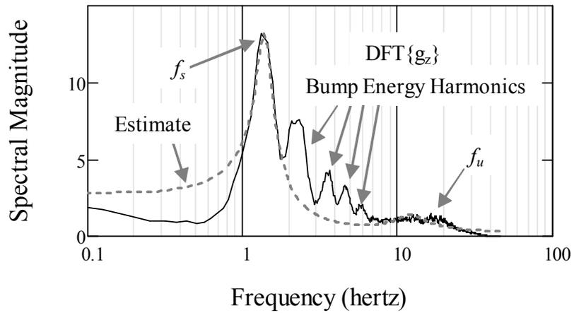
Figure 7. DFT of accelerometer output and an estimate of the equivalent quarter-car response
