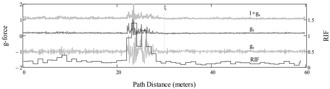
Figure 1. Accelerometer signals and RIF profile from a single traversal of speed bump at  $7 \text{ m} \cdot \text{s}^{-1}$
