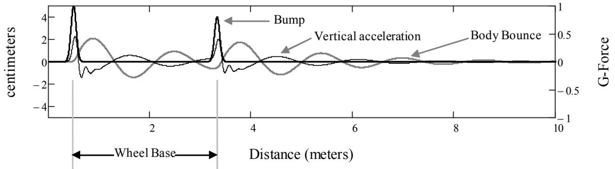
Figure 3. Simulated bump profile, vehicle body bounce response, and accelerometer signal
