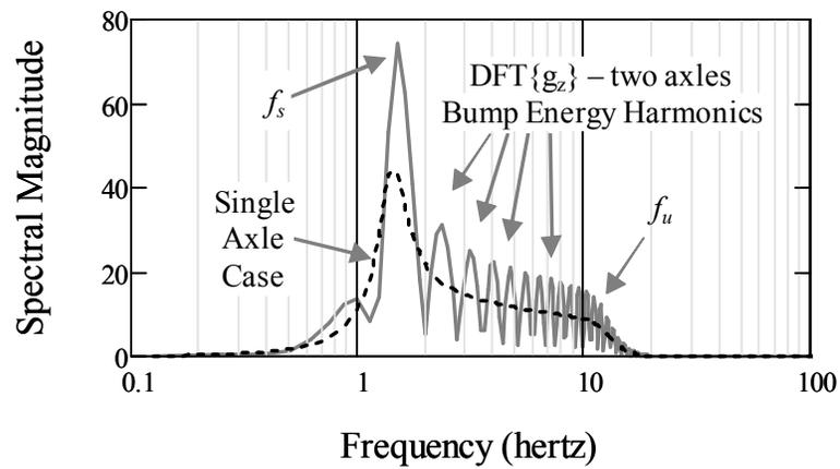
Figure 4. DFT of simulated accelerometer signal for single- and double-axle traversals
