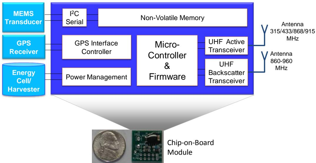
Figure 5: Typical architecture of a sensor based on existing RFID technology.
