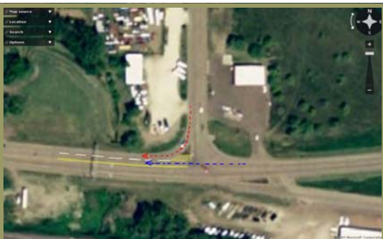
Figure 5: Example of Suggested Lane Striping
