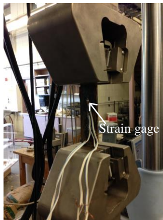
Figure I.3 Post-corrosion monotonic tension test
