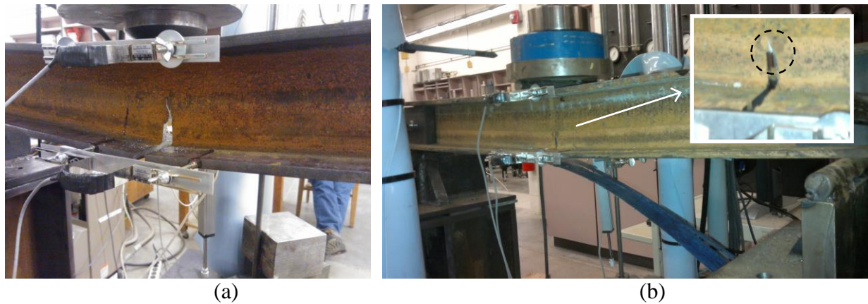
Figure II.9 Failure mode: (a) ductile fracture cracking; (b) CFRP-debonding
