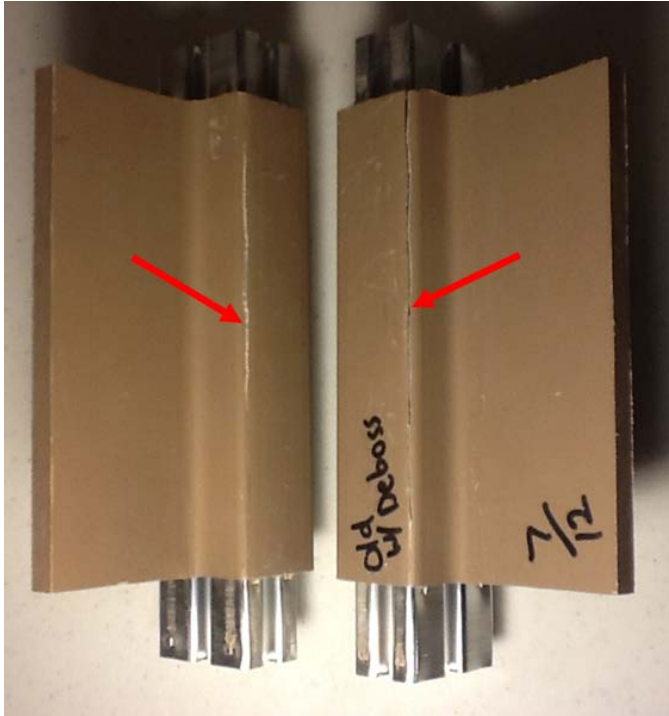
Figure 5.10 Cracks formed in specimens 7 (right) & 8 (left)
