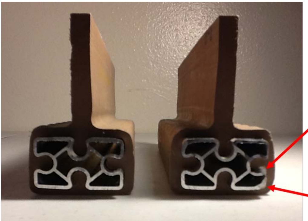
Figure 5.3 12-inch (a) specimen (left) vs. 12-inch (b) specimen (right) showing deformed aluminum that was blocked by push-through plate
