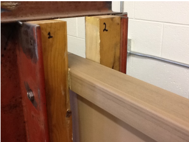
A) Greased wood lateral support inserts
