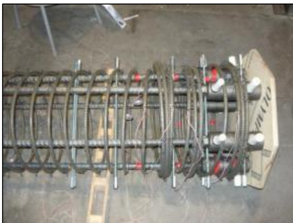
(a) Column end FGSS and overlapping spiral.
