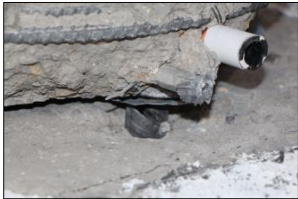
(c) Damage state at 9% drift ratio: spalling, exposed rebar cage, and fractured bar.
