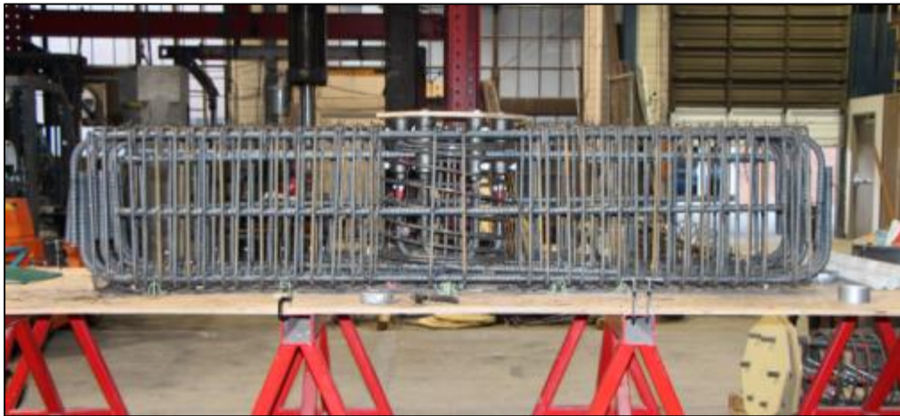
(b) Cap beam rebar cage.
