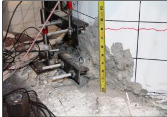
(b) Damage state at 6% drift ratio: cracks, spalling, and yield penetration.
