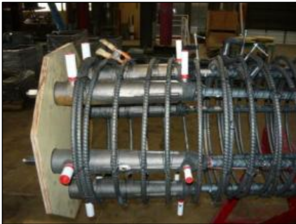
(a) Column end GGSS and overlapping spiral.
