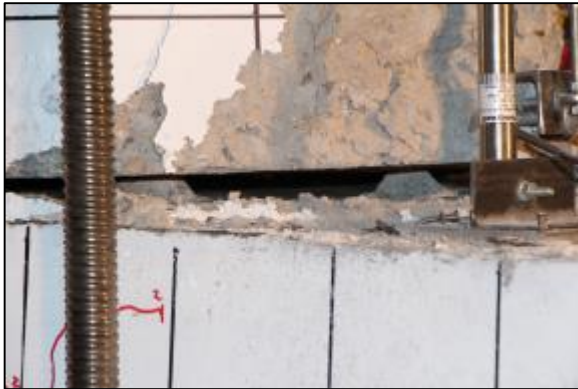
(c) Bar pull-out during 6% drift ratio.
