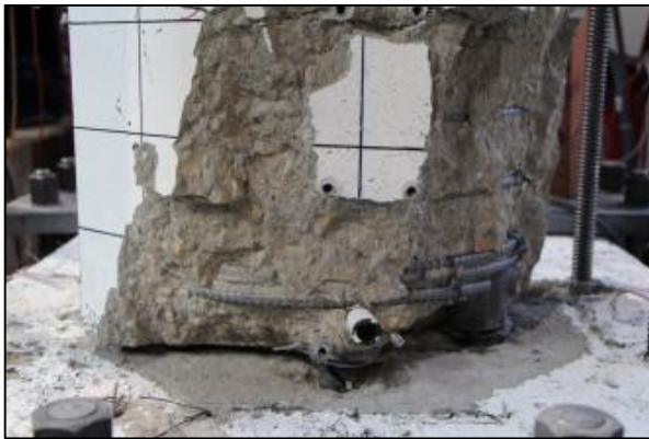
(c) Damage state at 9% drift ratio: spalling, exposed rebar cage, and fractured bar.
