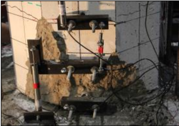
(b) Damage state at 6% drift ratio: cracks, spalling, and yield penetration.
