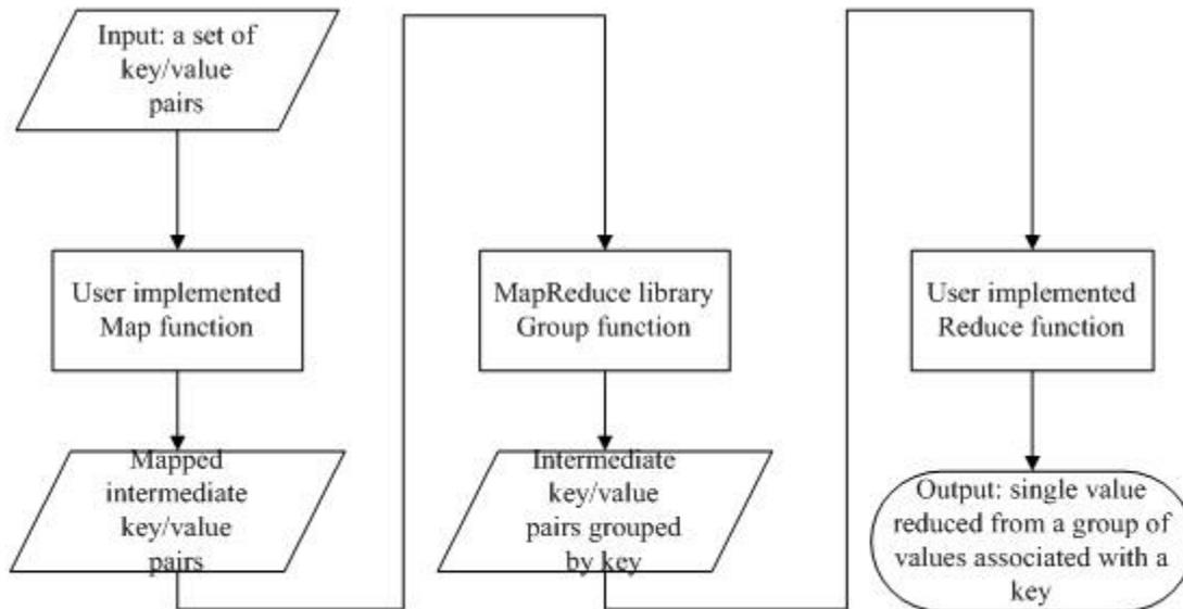
**Figure 2:** A typical MapReduce Computation Process
