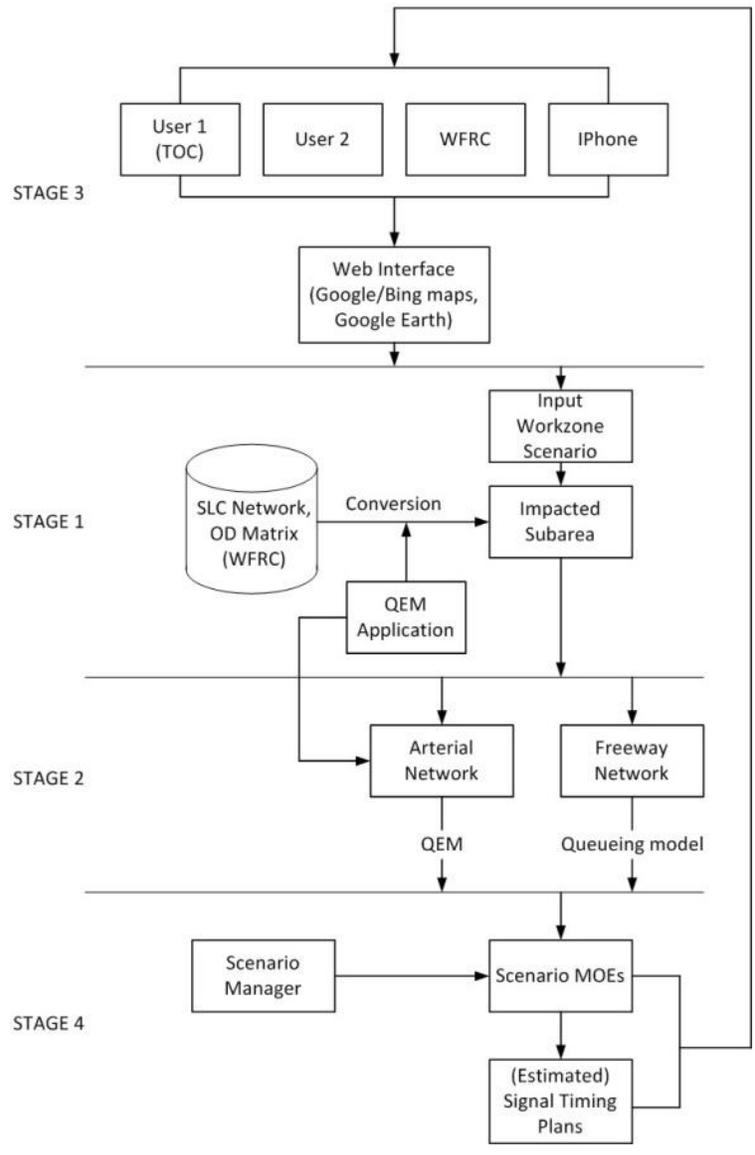
**Figure 1.1** Flow Process for Traffic Management Analysis and Work Zone Impact Estimation
