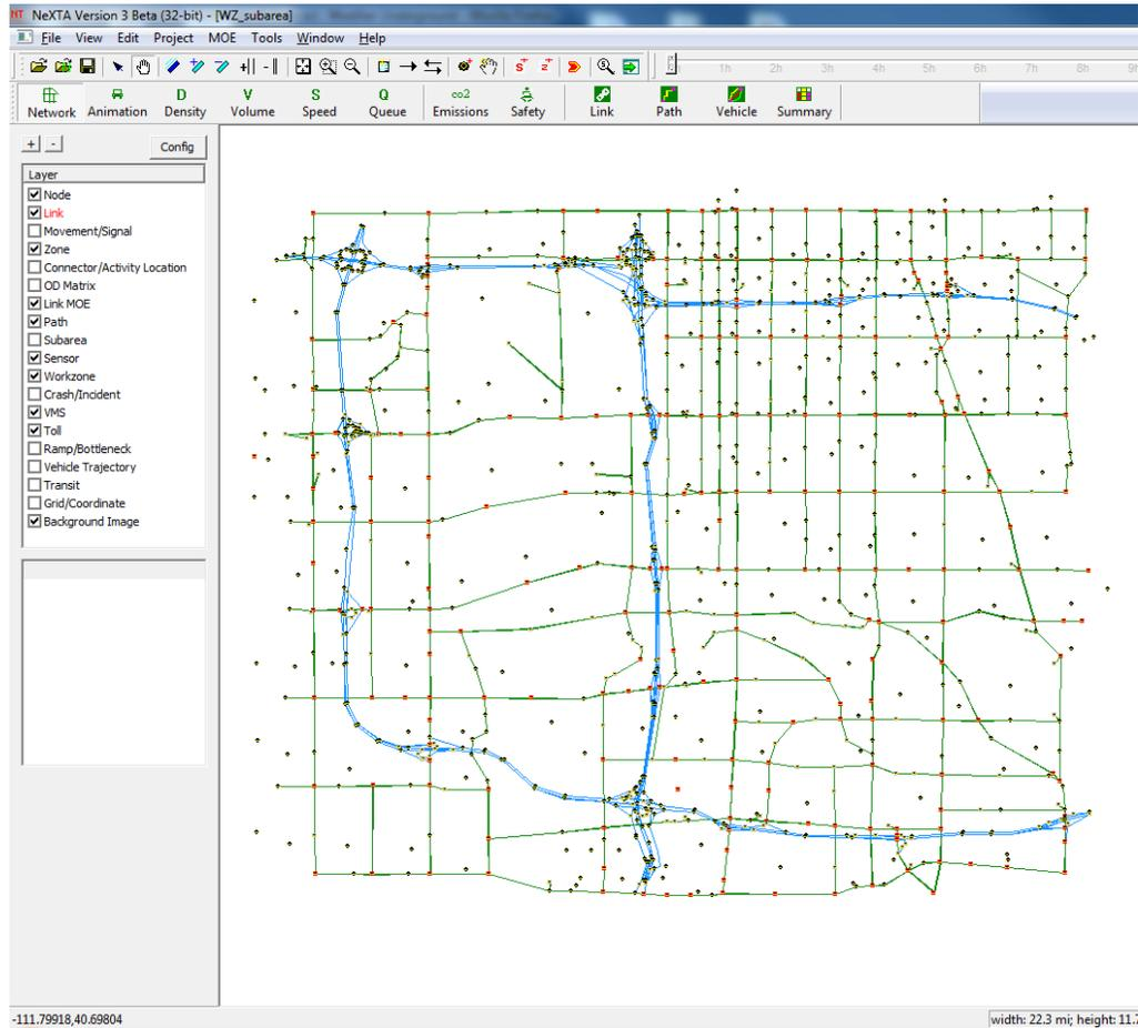
**Figure 6.10** Work Zone Subarea Network in NeXTA
