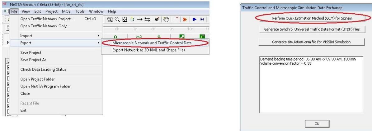
Figure 6.21 Starting QEM through NeXTA Interface
