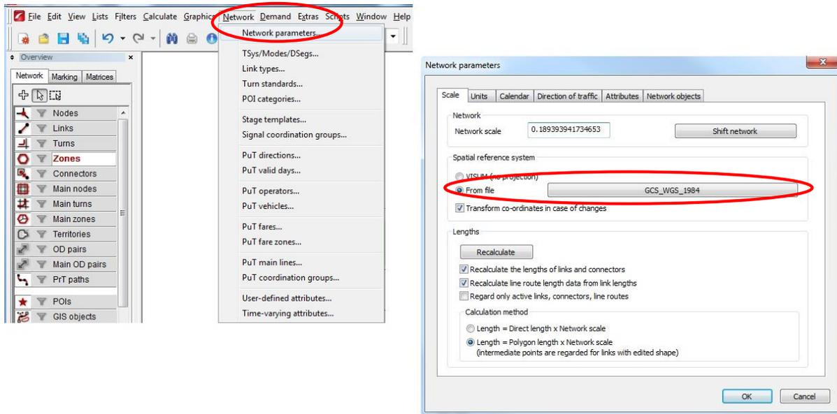
**Figure 6.4** Setting Map Projection System in VISUM
