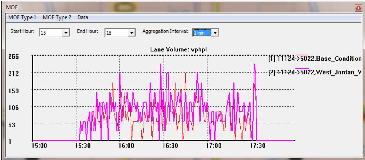
This plot shows the number of vehicles passing through this link (in vehicles per hour per lane) for both simulations (the red line represents the simulation without work zone, and the purple line represents the simulation with work zone conditions). We can show different MOEs by selecting different options in the MOE Type 1 menu, and smooth the data by adjusting the aggregation interval. Switching to the 15 minute aggregation interval produces the following plot.
