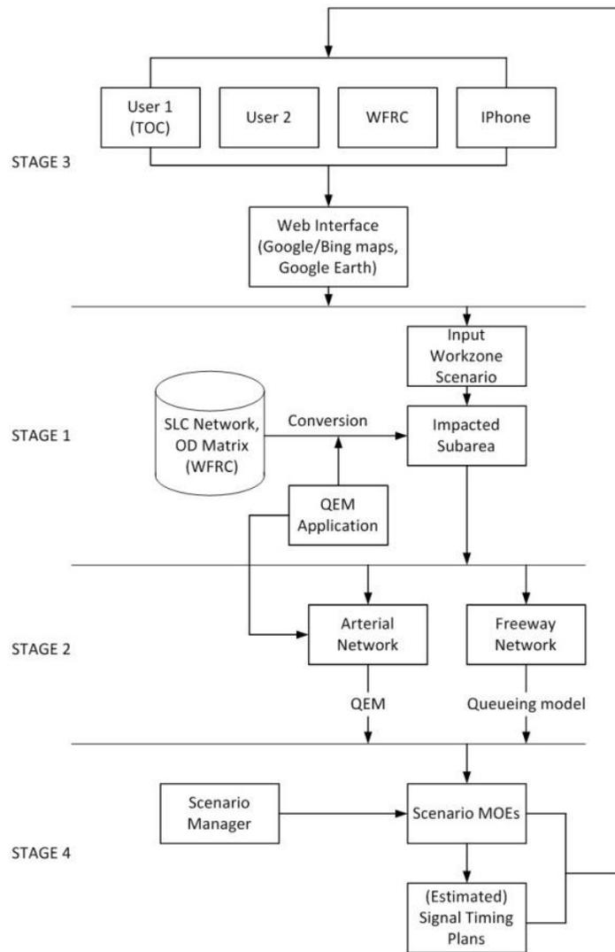
**Figure 4.1** Data Hub Workflow and Backend Simulation Engine
