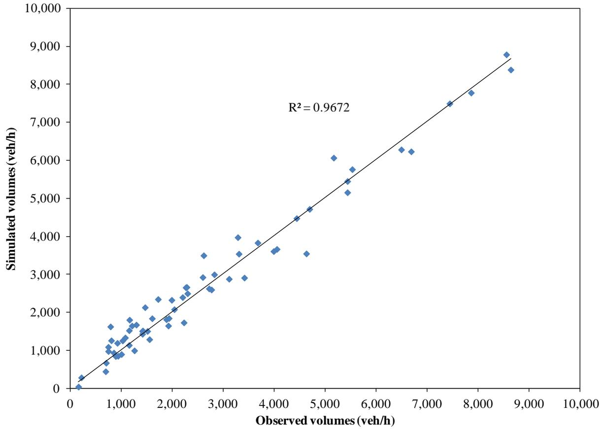
**Figure 7.3** SR 201 Test Case Network Validation
