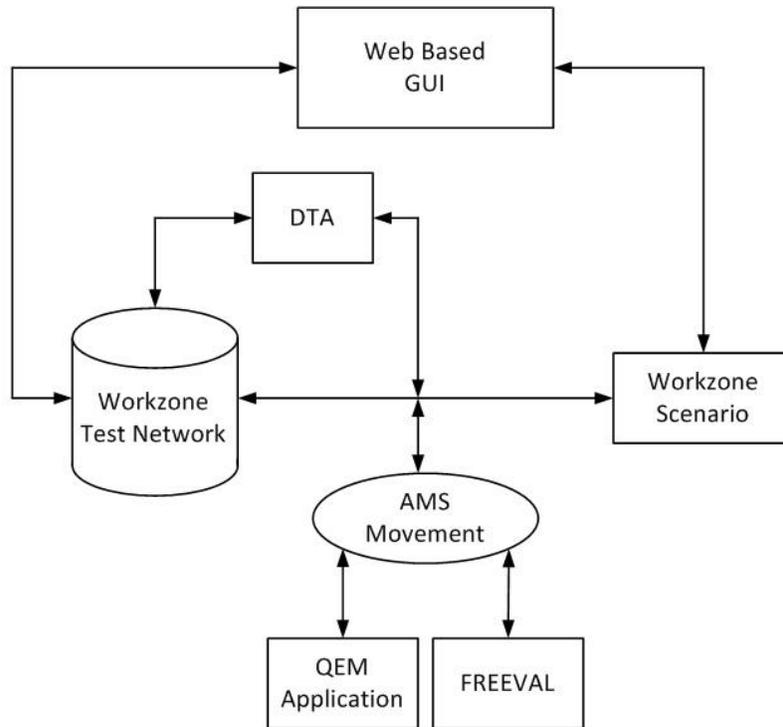
**Figure 6.2** Work Zone System Design
