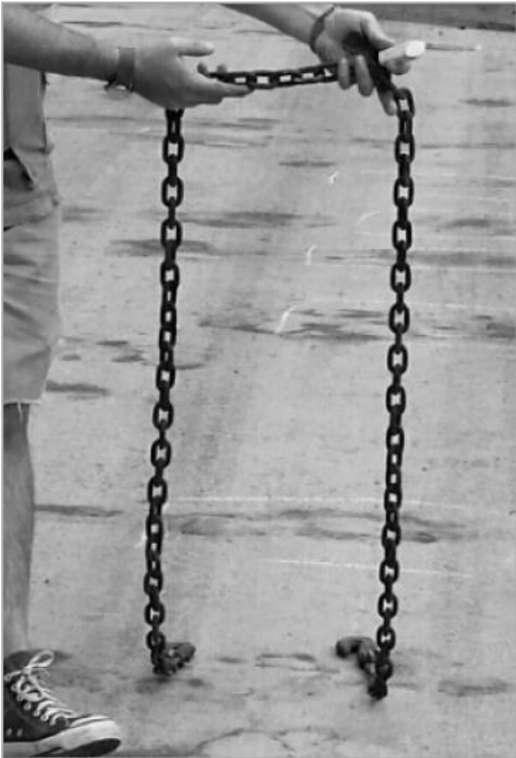
Figure 8.7 Chain drag test to detect delamination
