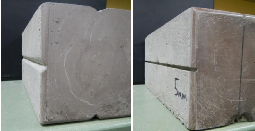
Figure 3.4 Concrete test prisms notches: (a) V-notch (b) Saw-notch
