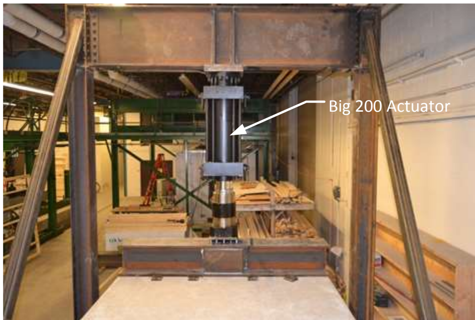
Figure 5.8 220-kip Actuator and Load Application Beam
