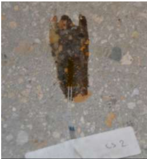
Figure 5.17 Strain Gage Attached to Top of Slab
