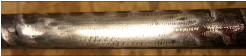
Figure 3.5 Deformed steel reinforcement with ribs ground down and sanded
