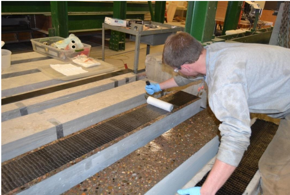
Figure 3.16 Hand-layup process of Tyfo SCH-41 CFRP sheets and beams 4 and 5
