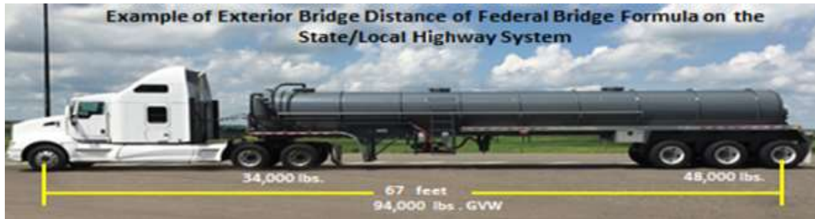
Figure 5: Illustration of Exterior Bridge Distance
