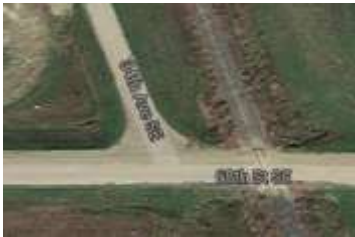
Figure 30: Typical County/Township Road Intersection Showing Tight Corner Radii
